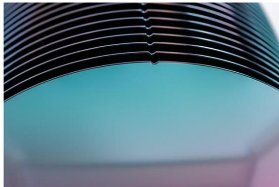
*Okmetic's UF-RFSi® is a tailored silicon substrate dedicated for thin film surface acoustic wave hybrid structures.*
